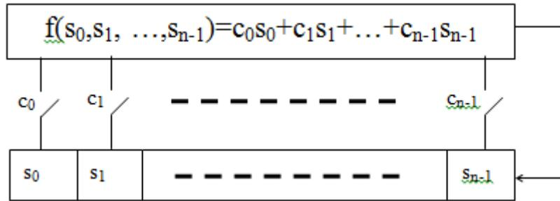
Figure (2) : Linear feed back shift register
