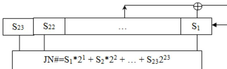
Figure (5) The jumps mechanism
