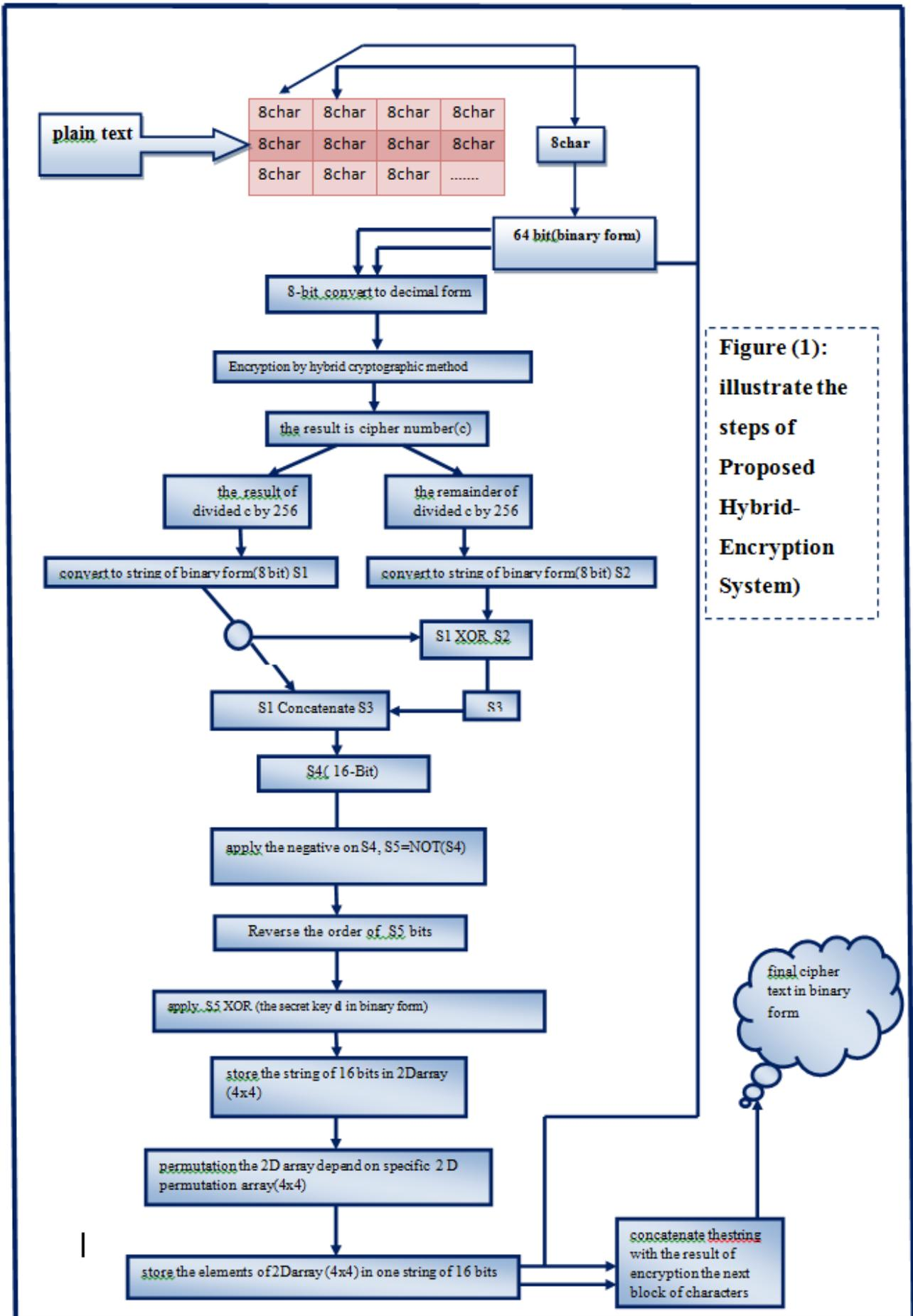
Figure (1): illustrate the steps of Proposed Hybrid-Encryption System)
