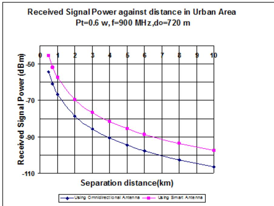
**Figure (3) The Received Signal Power against Distance Using Omnidirectional and Smart Antenna**
