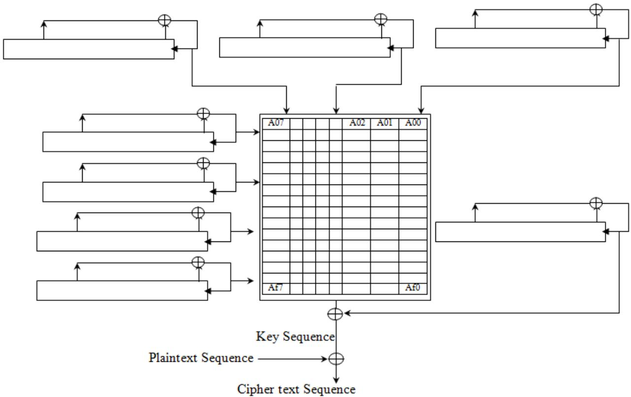
Figure (4) Cryptographic mechanism
